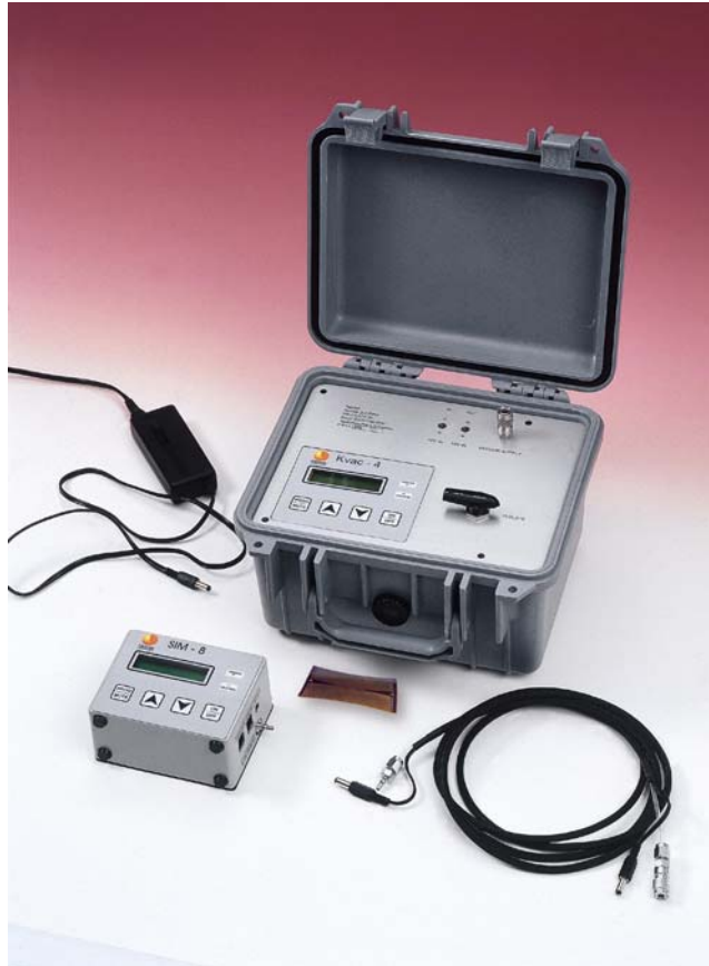
Figure 9: Comparative Vacuum Monitor System 2000 used for the high strain trials. The picture shows the larger field unit and the smaller laboratory unit.
