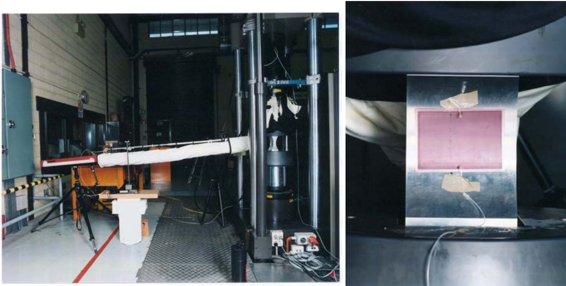
Figure 1: Large specimen set-up with laser holography on rear-face (left) and CVM system sensor (right) on front face. The reason for the shroud is to reduce external light when holographic plates are being exposed.
