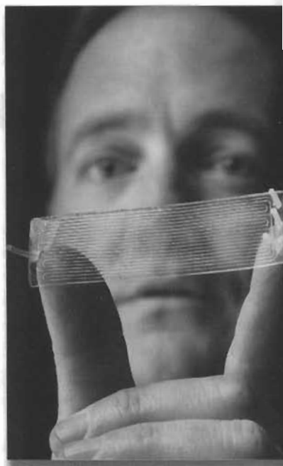
Dennis Roach with a Comparative Vacuum Monitoring (CVM) sensor that shows galleries etched into the sensor's underside. Photo courtesy of Randy Montoya.
